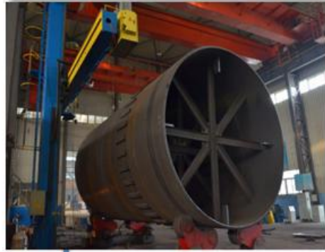
埋弧自动焊 (焊缝UT) Submerged-Arc Welding ( UT)
