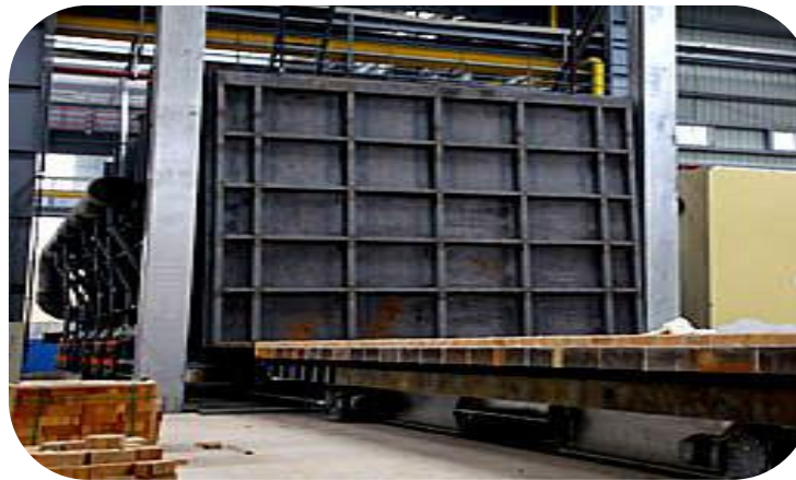
◆ 3X6.3m Heattreatment Furnace
