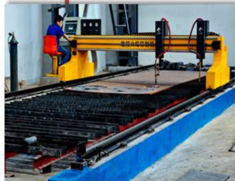
数控下料切割 CNC Cutting Machining
