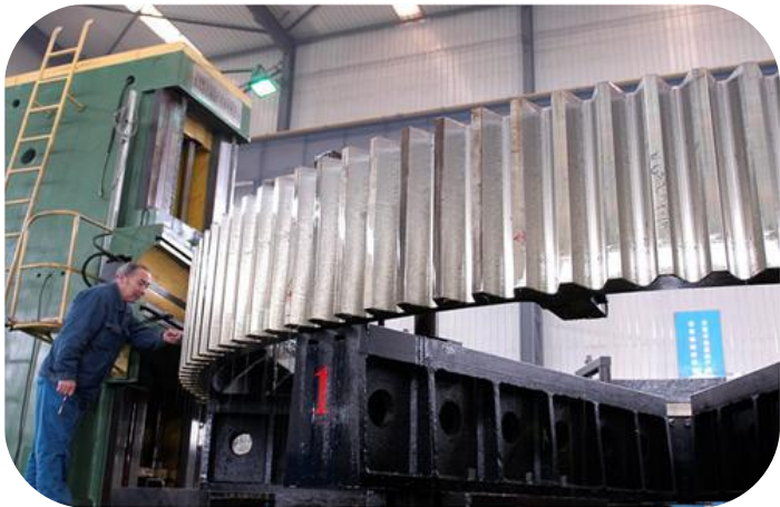
Girth Gear Testing
